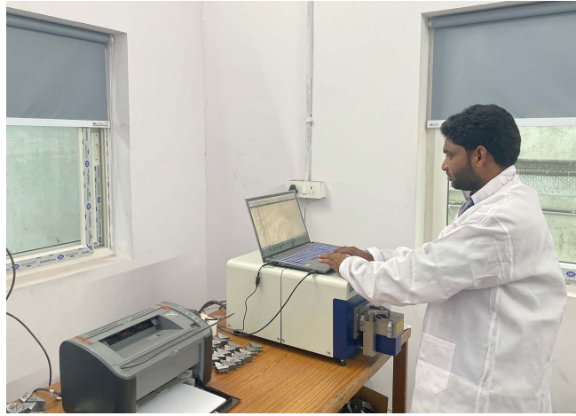
Spectrometer for testing of chemistry of Raw Materials and Finished goods in house Laboratory.
