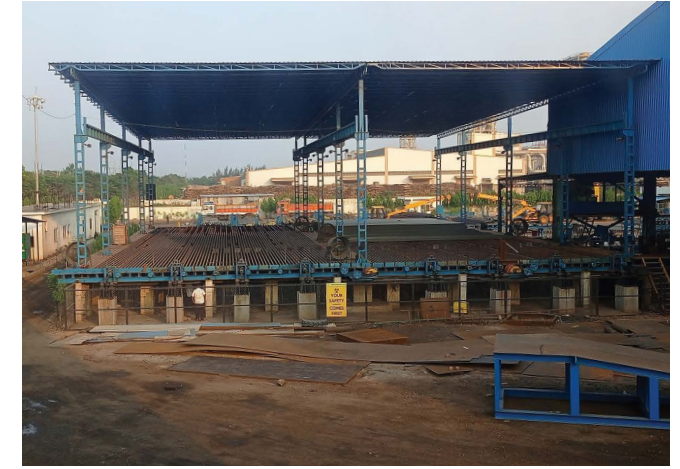
Cooling Bed of 30mtrs x 45Mtrs for natural cooling and normalizing the hot rolled Steel structural and Round bars of different sizes.
