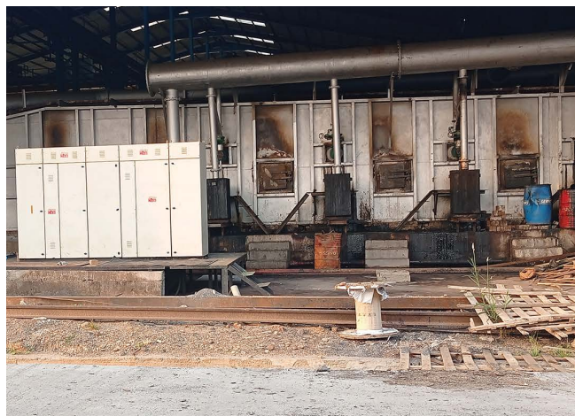
30Mtrs(l) x 6Mtrs(w) – with holding capacity of 350MTs and with 15MTs/Hr rate of heating, Coal Gas fired Reheating furnace.
