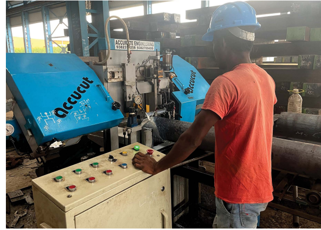
Band saw Cutting Machine assemblies for the customized size/length cutting of the Rounds of sizes ranging from 85mm dia. to 240mm dia.
