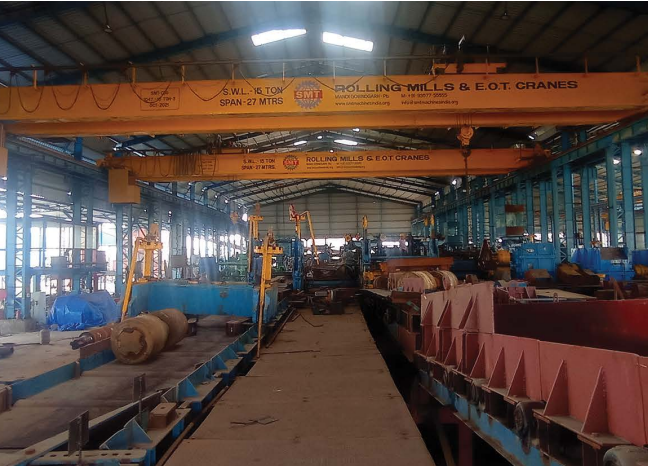
EOT Cranes assemblies. of 15MTs capacity with 27mtrs Span
