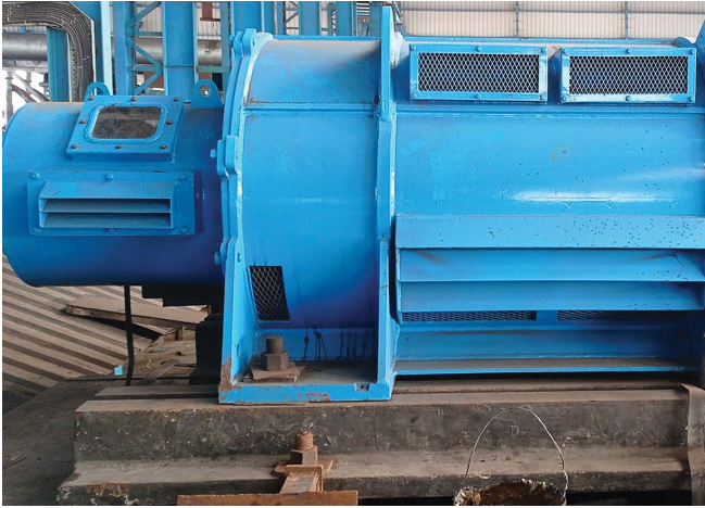
26" CRS Rolling Mill -Rd. Gear Box- Pinion Gear Box assembly with 3Hi-Rolling Mill stand Assembly – stage 1 driven with 2000HP A.C Slipring Motor- stage 1
